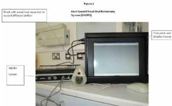
Figures 1: Kent Special Nasal Ratiometry System (SNORS)
